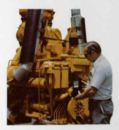
Low daily maintenance means low operating costs and high machine productivity. Grease points are eliminated on the basic tractor and reduced on ripper and dozer for fast, economical service. Fast-check sight gauges are used for hydraulic oil, power train oil and coolant levels. Spin-on oil filters provide quick, contaminant-free filter replacement. Spin-on fuel filters and fuel priming pump are located inside the service door on the back of the fuel tank for easy servicing.
