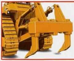
Rugged Cat Rippers are available for added machine versatility. Hydraulic tip adjustment cylinders vary shank angle to aid penetration and help lift and shatter rock . . . for high productivity and long shank life. Streamlined and narrowed ripper frame improves single shank performance through minimum clogging and slab retention. Standard single shank pin puller lets operator adjust shank length from the seat. Multishank ripper allows use of one, two or three shanks, depending on job conditions.
