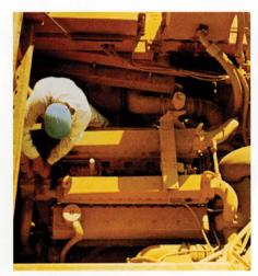
Rear section of the service deck tilts forward to open a completely accessible engine compartment — giving mechanics an uncluttered work area around the engine. A brace holds the door upright. And both the engine oil dipstick and the oil filler spout can be reached without raising the deck.
