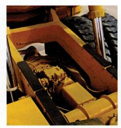
In-frame service of engine and pump groups is convenient with unrestricted access. Raise the dump body and insert self-storing retaining pins for access to torque converter, drive shaft, transmission and differential.
