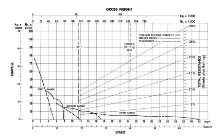
To determine gradeability performance: Read from gross weight down to the % of total resistance. [Total resistance equals actual % grade plus 1% for each 20 lb./ton (10 kg/t) of rolling resistance]. From this weight-resistance point, read horizontally to the curve with the highest obtainable speed range, then down to maximum speed. Usable rimpull will depend upon traction available and total weight on drive wheels.
