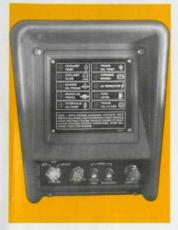
Operator's compartment features Electronic Monitoring System (EMS) for status check of important machine systems with three levels of warning.
