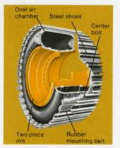
Caterpillar steel shoe Beadless Tires . . . an optional arrangement that can provide increased tire life, reduced total tire costs and greater machine productive capabilities in abrasive applications and load-and-carry. Steel shoes help protect against sudden tire failure from rock cuts and short tread life from abrasion. They bolt directly to a replaceable mounting belt. Oval air chamber carcass is helically wound with tough steel cable for strength and protection.
