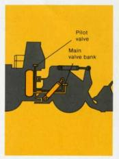
Pilot-operated control valves provide control . . . plus ease of operation. Hydraulic control levers are in a console to the operator's right. When the levers are engaged, pilot hydraulic pressure actuates the main control valve to meter oil flow to the corresponding lift or tilt cylinders, while the remote pilot valve maintains a constant pressure. No reaction delay, and lift arms and bucket can be inched and feathered with accuracy.
