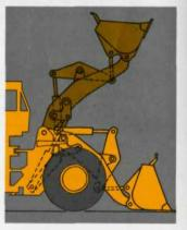
High breakout force on the 992C is due to the mechanical advantage of the Z-bar linkage geometry and an effective, efficient use of the hydraulic system forces. With this linkage, the bucket's dump velocity decreases near the end of its dump motion, resulting in reduced dump shock.
