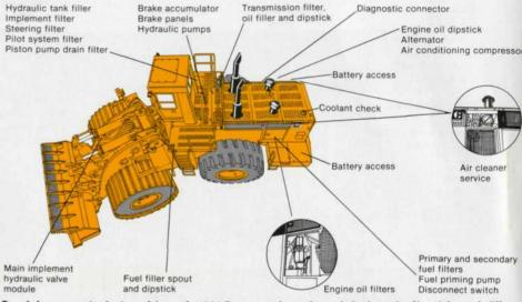
Servicing ease is designed into the 992C:
