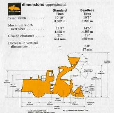
992C buckets provide exceptional flexibility in matching the machine to job conditions. All are welded construction, abrasion-resistant steel, with high-strength material used in side plates, side cutting bars and bucket shells. They feature a tapered floor design of approximately 7°, with box-sectioned reinforcing material placed under the floor for increased structural strength.
