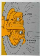
Four-wheel oil disc brakes have 4748 sq. in/30 635 cm² of braking surface per wheel. Each brake has nine discs and ten plates cooled by oil for long life. They are completely sealed and require no adjustment.
