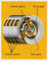
Power shift transmission is designed for tough work . . . with big clutch packs surrounding planetary gear sets. Hydraulic modulation cushions clutch engagement for on-the-go shifting. Planet gears spaced 120° apart spread torque loads for longer life. Oil cooling and lubrication reduce heat and wearing friction.
