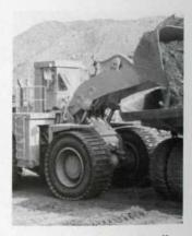
Caterpillar steel shoe Beadless Tires are available in all wheel or front wheel arrangements.
