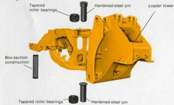
Loader tower and box-section main frame resist twisting and bending on rough ground. Two hardened-steel pins couple the front and rear frames. Both pins ride in double-tapered roller bearings. Bucket lift arms pins and hydraulic cylinder mounting pins are supported on both ends by steel plates in the loader tower, rather than on a single end as with cantilever mounting.
