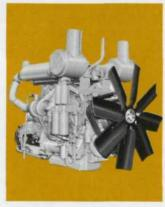
Cat 3412 diesel Engine has excellent response — the kind of response necessary for the stop and start operation of a loader. Twin turbochargers pack more air into cylinders for more power. Individual, interchangeable injection pumps for each cylinder require no adjustment. Large injection valve openings help prevent carbon build-up, even during idling.
