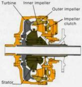
Variable capacity torque converter lets operator apportion power between hydraulics and drive train to match job requirements. Two impellers in the converter are the key. The inner impeller always rotates at engine speed. The outer impeller connects to a clutch which can gradually engage the impeller to send more or less power through the converter for more or less rimpull. The operator can select appropriate setting for the job, from a soft setting to full match.
